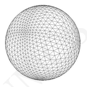
Fig. 8. Unstructured mesh on a sphere
