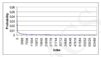
Fig. 1. Probability distribution of indexes generated by LZSS method during compression of file "xplik"
