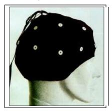
Fig. 2. Mindset MS-1000 EEG system Electo-Cap
